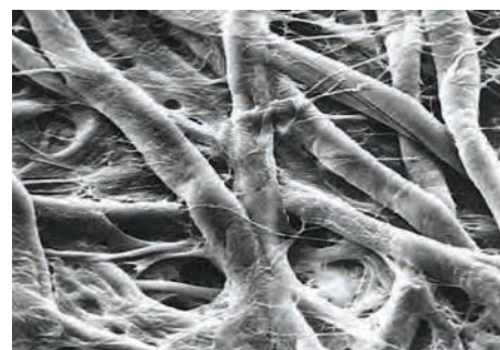
Whatman cellulose filter papers exhibit particle retention levels down to 2.5 µm.
